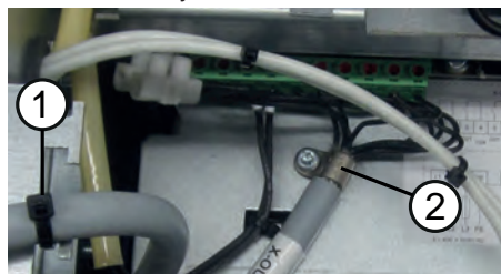
Shielding digital outputs line 1 Strain relief by cable ties 2 Earthing clip
