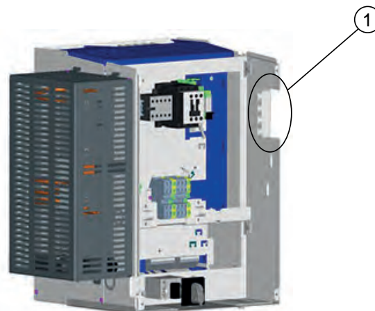
Wiring 1 Cable brakes, cable brake resistance, cable motor temperature monitoring, cables X-ENC15, X-ENC8, X-MON
